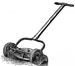
A cylinder (reel) mower from 1888 showing a fixed cutting blade in front of the rear roller and wheel-driven rotary blades.
